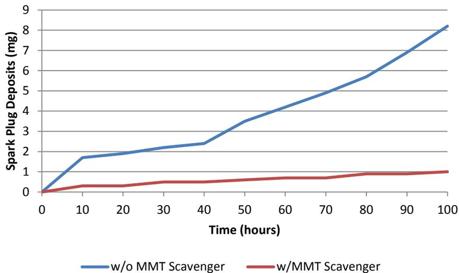
Just how effective is our alkyl halide-catalyzed MMT scavenger + detergent? This graph shows test results of quantified spark plug deposits in two test engines, both running gasoline that was heavily dosed w/No-Rosion Octane Booster at 6 bottles per 20 gallons. As you will note, the one inclusive of our MMT scavenger saw average plug deposits of about 1.0 mg versus over 8.0 mg on plugs without the MMT scavenger.
